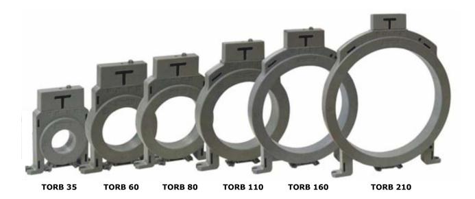
Toroidal current reducers to be combined with the By11600, type B residual current relay. Made up of a special magnetic core which allows the detection of fault currents with a value of a few mA AC / DC.
